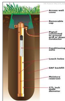
Gambar 1 Metode Driven Rod
