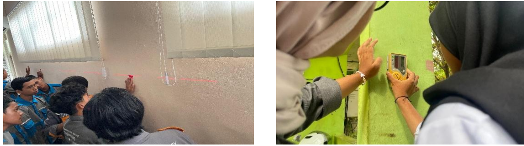
Gambar 7. Praktik LKS 3 Rotating Laser dan Marking Level
