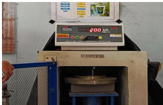
Gambar 16. Proses Pengujian Kuat Tekan Paving Block Normal
