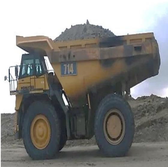
Gambar 3 Alat Angkut *Off Highway Dump Truck* Komatsu HD785-7
