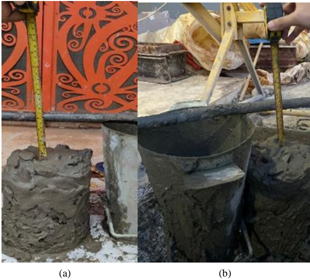
(a) (b) Gambar 6. Pengujian Slump (a) Slump Beton Normal (b) Slump Beton PET Variasi 0,30%
